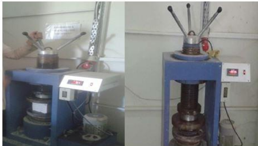
Fig. 2. Compressive strength test
