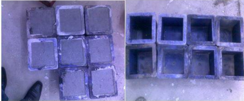
Fig. 1. Filled up Concrete Cubes
